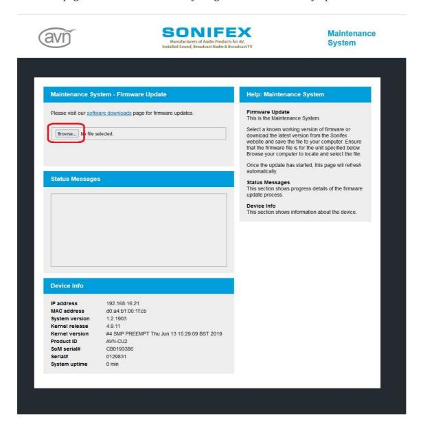
If your unit is already showing the maintenance screen on the display and asking for a firmware update, the ip address you need to connect to should be shown towards the top of the display, this is what you need to type into your web browser followed by :8080
