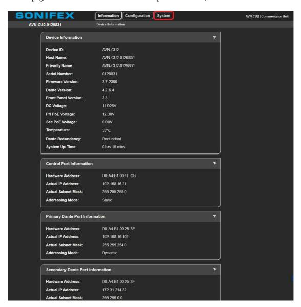
This will open the page from which you can upgrade the firmware of the unit. At the top of the screen click "Update", a message will appear informing you the unit will reboot.... Click continue if you wish to upgrade the firmware. After approximately 20 seconds the unit will reboot into the Maintenance System webpage.
